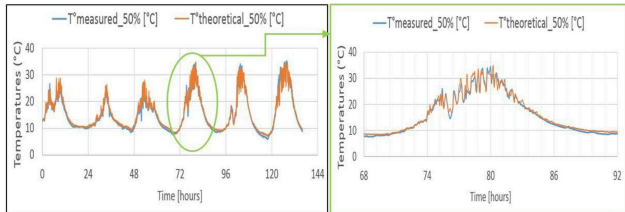
Fig. 6. Comparison between theoretical and measured temperatures ( $\sigma_{occ} = 50\%$ ).
