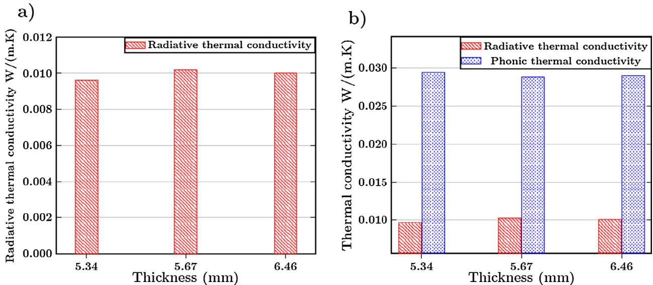
**Fig. 10.** (a) The radiative thermal conductivity as a function of samples thickness, (b) thickness effect on the radiative and phonic thermal conductivity.
