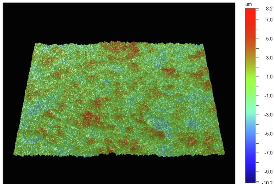
**Fig. 3.** 3D image of the new formwork roughness profile.**Table 2**
