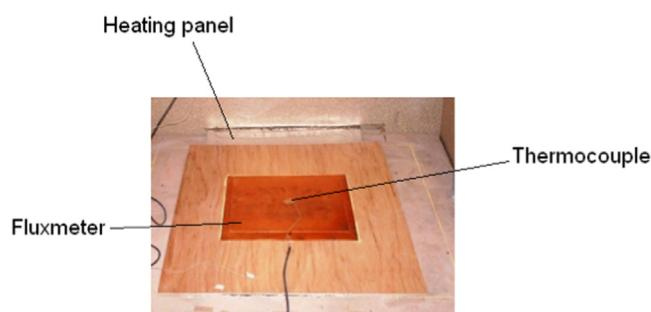
Fig. 2. Detail of the device of measure.
