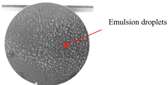
**Fig. 4.** Surface state after spraying on the formwork.
