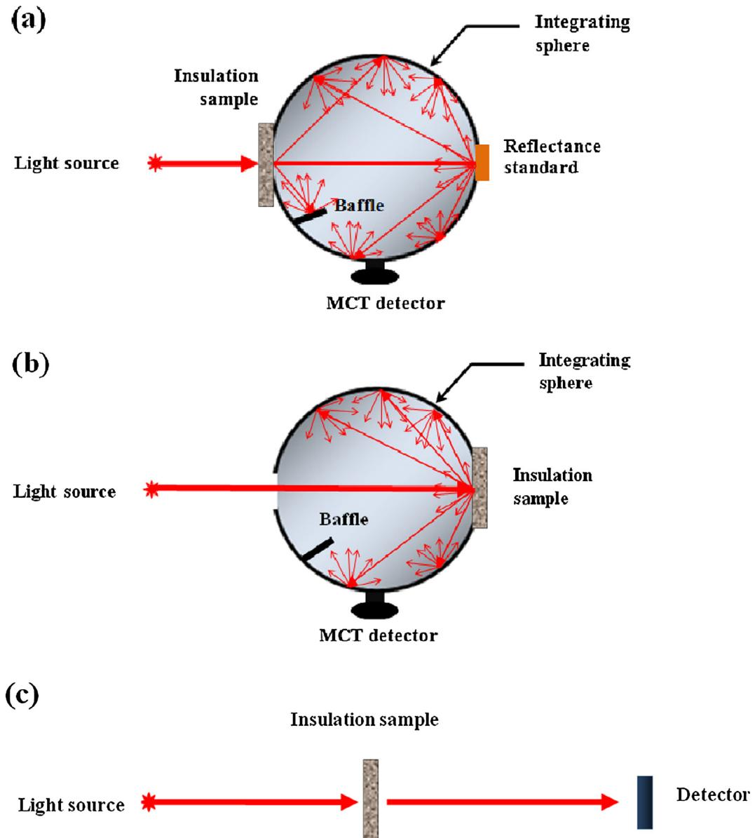
Fig. 2. Investigation mode, (a) procedure for measuring hemispherical transmittance  $T_{\lambda,\text{th}}^{\text{dh}}$ , (b) reflectance  $R_{\lambda,\text{exp}}^{\text{dh}}$  and (c) direct transmittance  $T_{\lambda,\text{th}}^d$ .
