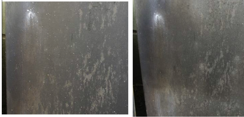
Fig. 15. Micrographs both before and after storage of sprayed oil 4.
