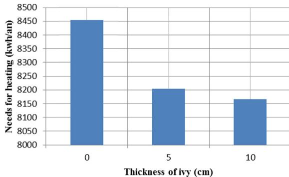
Fig. 11. Comparison for heating with or without ivy.
