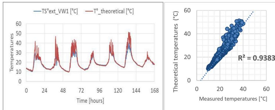
**Fig. 9.** Comparison of theoretical and measured temperatures.
