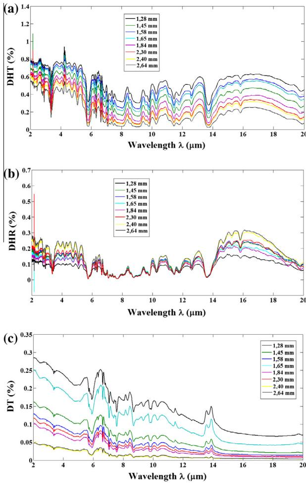
**Fig. 5.** (a) DHT<sub>exp</sub>, (b) DHR<sub>exp</sub> and (c) DT<sub>exp</sub> of polyester batting versus wavelength for different thicknesses.
