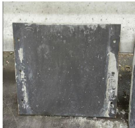
**Fig. 10.** Formwork obtained with mineral oil.
