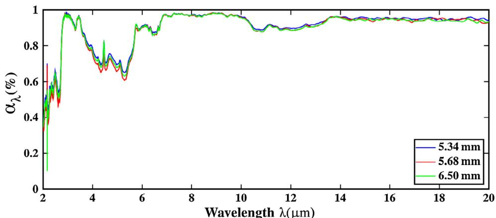
Fig. 5. Absorptance of insulation based on recycled textile versus wavelength for different thicknesses.
