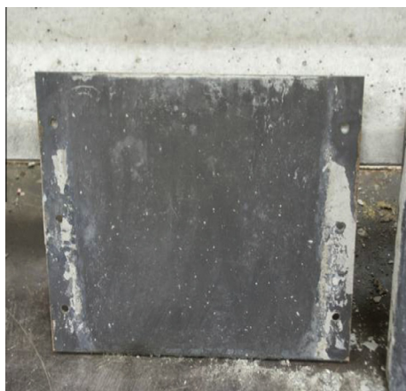
Fig. 10. Formwork obtained with mineral oil.
