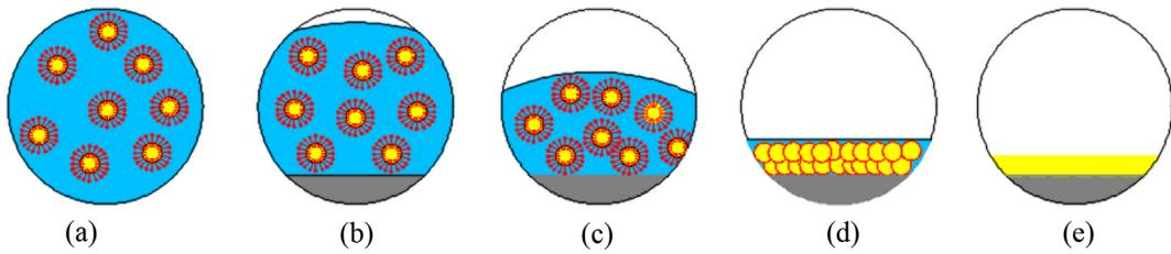
**Fig. 10.** Evolution diagram of the direct emulsion over time.
