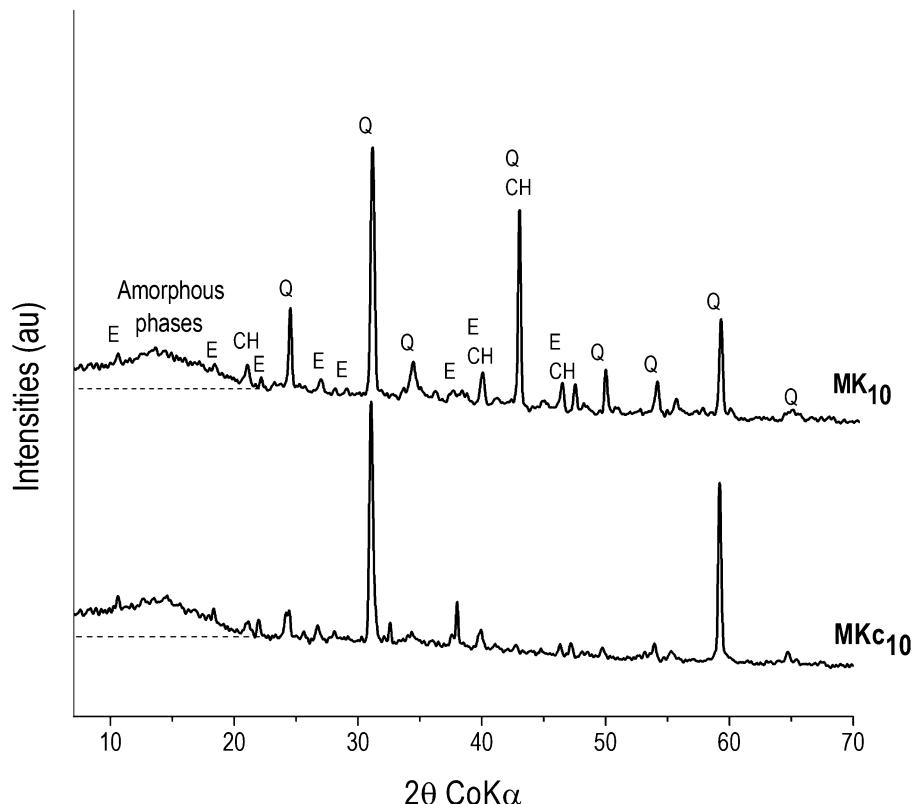
**Figure 9.** XRD patterns of MK<sub>10</sub> and MKc<sub>10</sub>: CH (Portlandite), E (Ettringite), and Q (Quartz).
