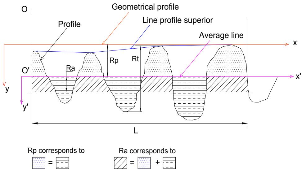
**Fig. 2.** Scheme of the roughness profile (height vs. length).**Surface Stats:**
