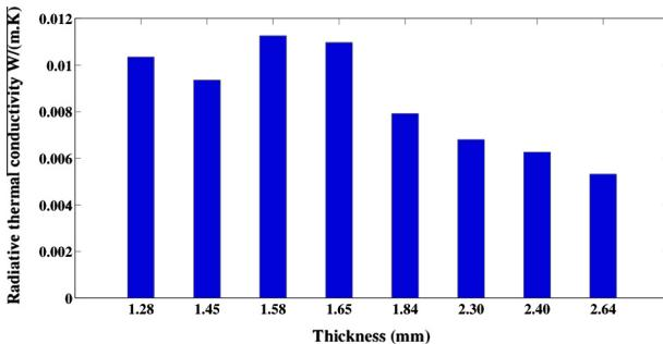
**Fig. 12.** Thickness effect on the radiative conductivity and the phonic conductivity with a fiber diameter of 31 μm.
