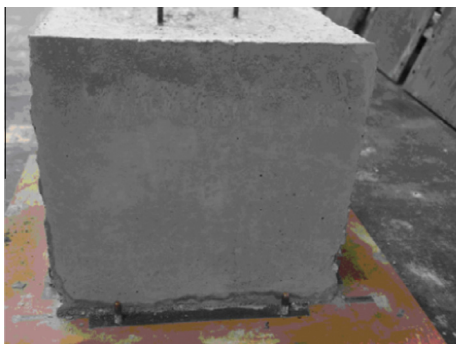
Fig. 7. Facing obtained with vegetable oil.
