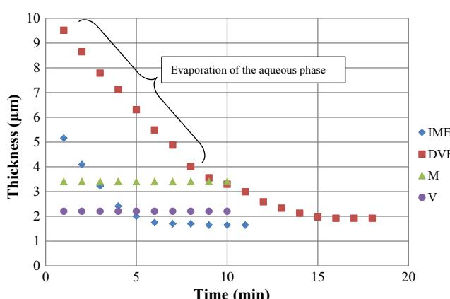
Fig. 7. Water evaporation kinetics for the deposited emulsions.
