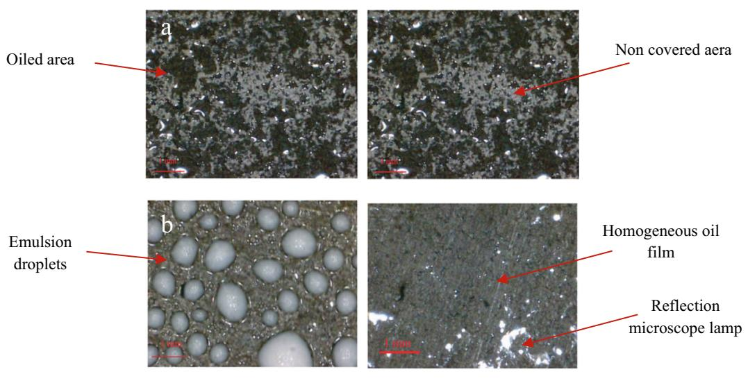
**Fig. 6.** Film micrographs after spraying (a) the V oil and (b) the DVE emulsion.
