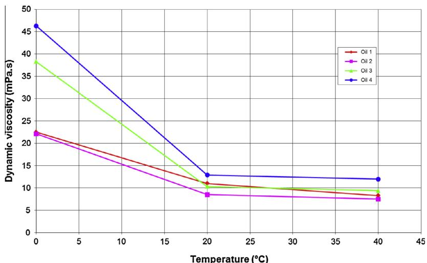
**Fig. 5.** Variation of dynamic viscosity according to temperature.
