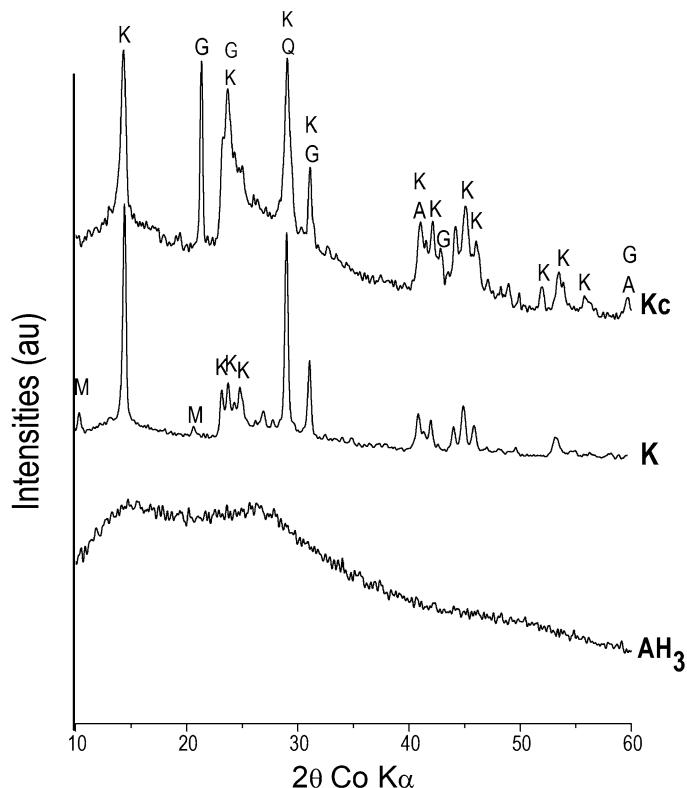
**Figure 1.** X-Ray Diffraction patterns of starting materials K, Kc and AH<sub>3</sub>; K: Kaolinite; A: Anatase; Q: Quartz; G: Gibbsite; and M: Muscovite.
