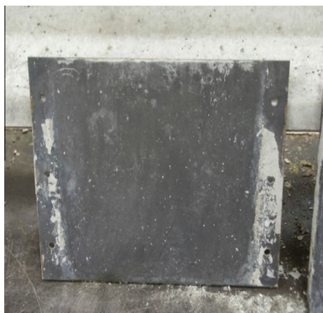
Fig. 10. Formwork obtained with mineral oil.
