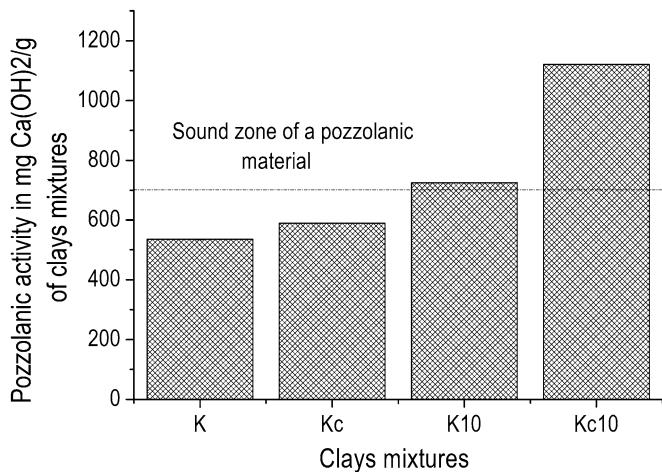
**Figure 4.** Pozzolanic activity by Chapelle test of clays (K and Kc) and of mixtures clays—10 wt% amorphous aluminum hydroxide (K<sub>10</sub> and Kc<sub>10</sub>).
