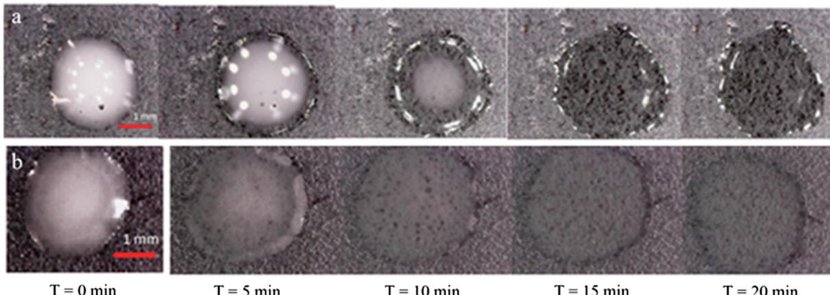
**Fig. 5.** Evolution of a drop of (a) DVE and (b) IME emulsions during the latency period.
