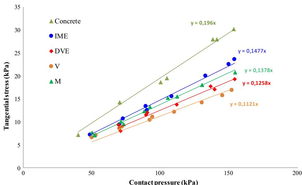
**Fig. 9.** Dynamic friction constraints according to the pressure ( $v = 0.84$  mm/s).
