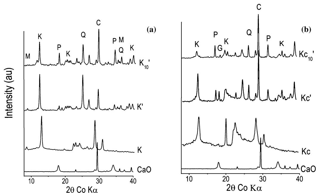
**Figure 6.** XRD patterns of materials before and after the Chapelle test: (a) CaO, K, K' and K<sub>10</sub>'; (b) CaO, Kc, Kc' and Kc<sub>10</sub>' for which K: Kaolinite; Q: Quartz; C: calcite; M: Muscovite, G: Gibbsite and P: Portlandite.
