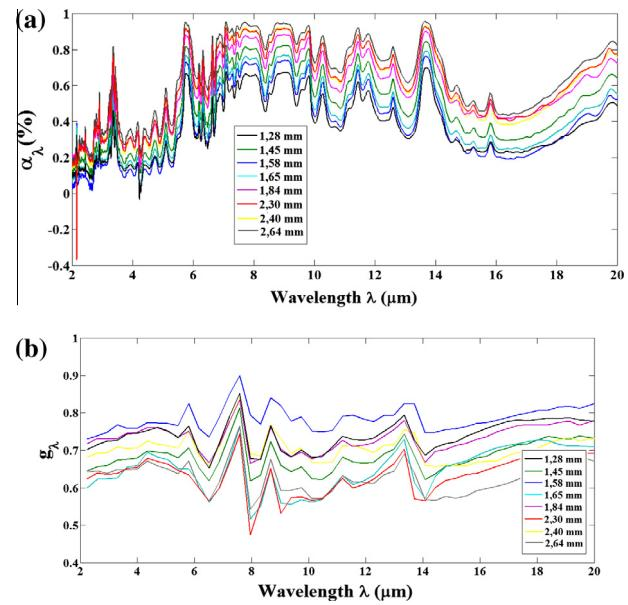
**Fig. 9.** (a) Absorptance of the polyester batting versus wavelength for different thicknesses and (b) the phase function versus wavelength for different thicknesses.
