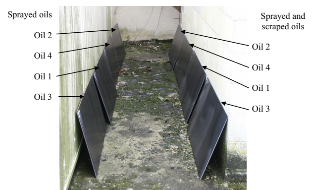
Fig. 11. Formwork surface storage zone.
