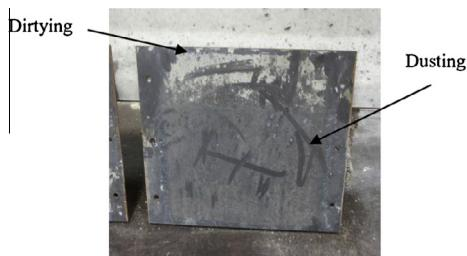
**Fig. 9.** Formwork obtained with vegetable oil.
