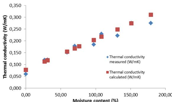
Fig. 8. Comparison between thermal conductivity measured and calculated.
