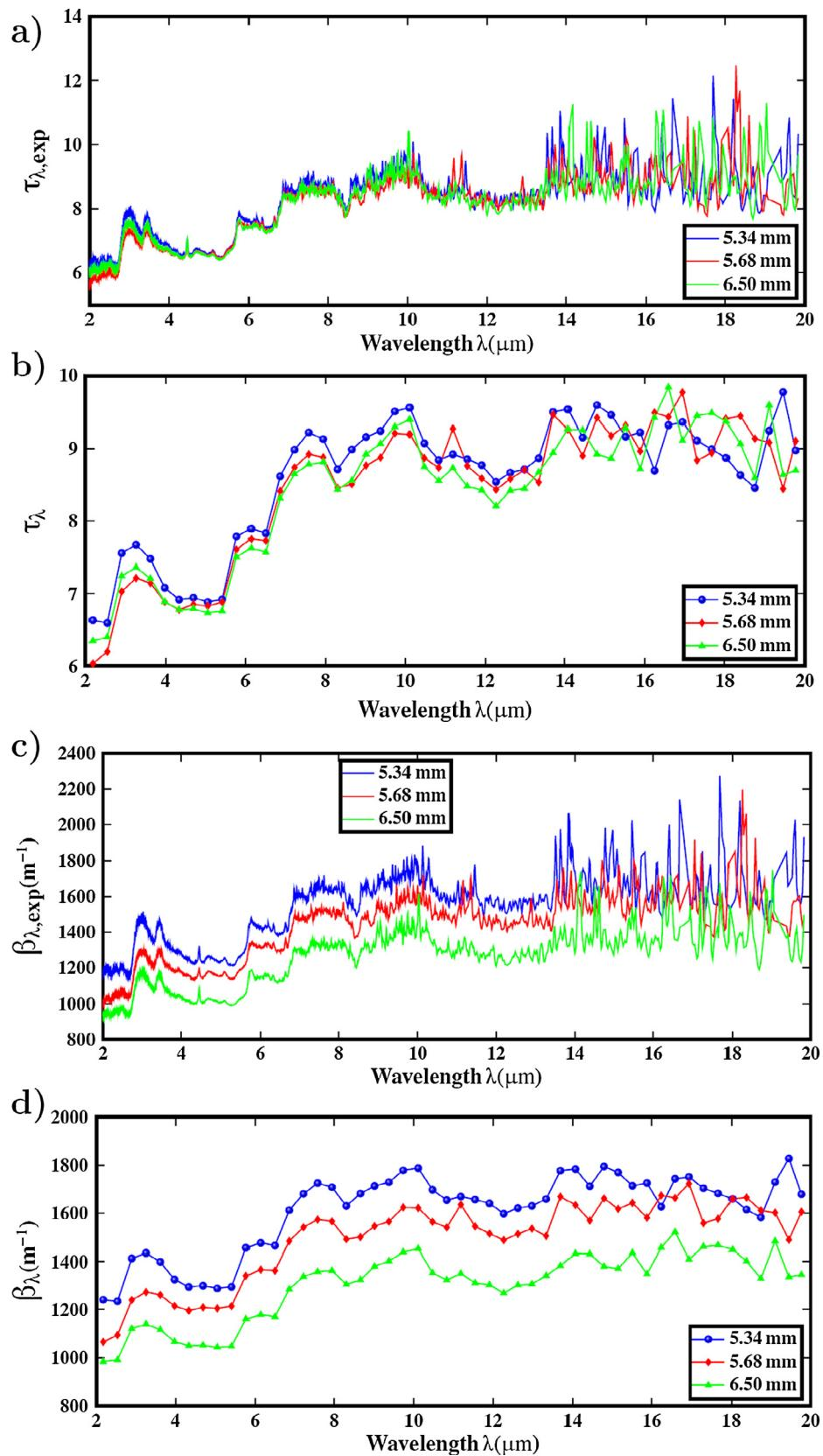
**Fig. 4.** Radiative properties of insulation material based on recycled textile versus wavelength for different thicknesses, (a) identified optical thickness, (b) calculated optical thickness, (c) identified extinction coefficient and (d) calculated extinction coefficient.
