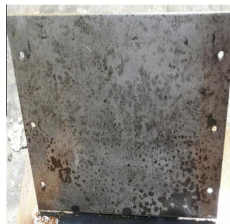
**Fig. 3.** Used formwork surface.
