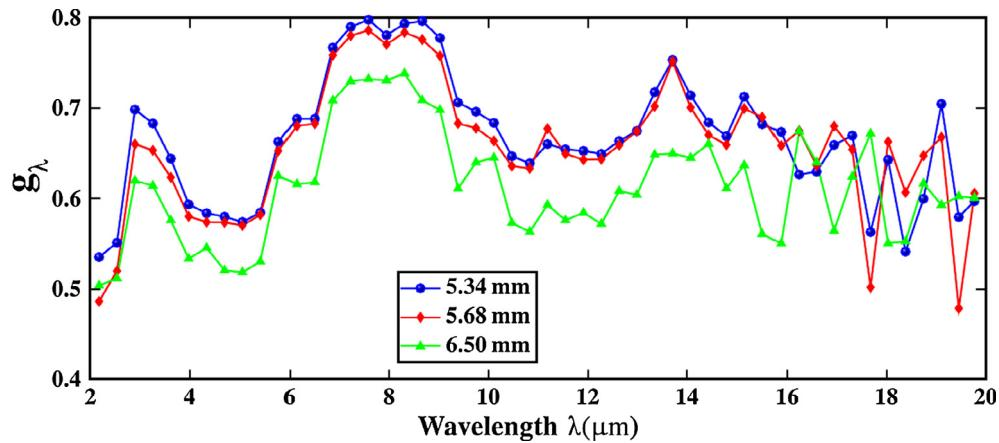
Fig. 6. Phase function versus wavelength for different thicknesses.
