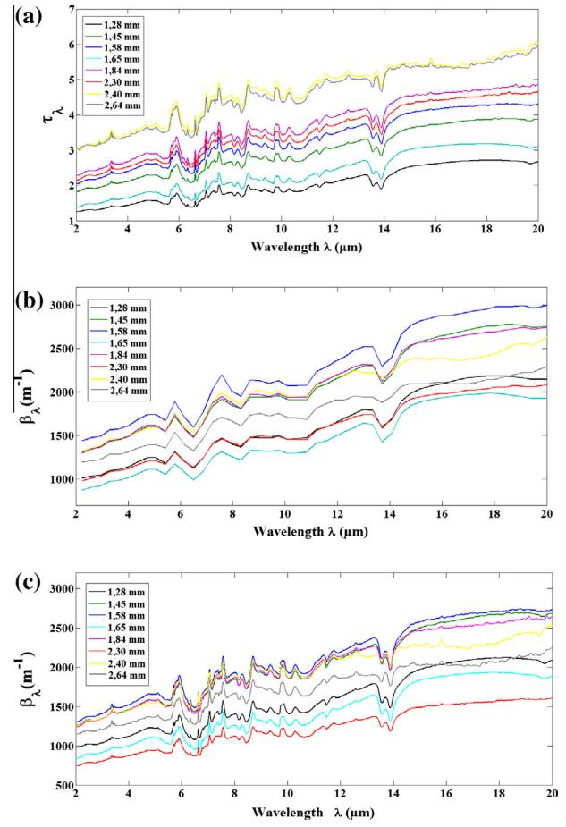
**Fig. 6.** Radiative properties of polyester batting versus wavelength for different thicknesses: (a) optical thickness of polyester batting, (b) identified extinction coefficient, and (c) calculated extinction coefficient.
