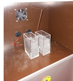
Fig. 2. Twisted pair in the breakdown voltage measurement device.
