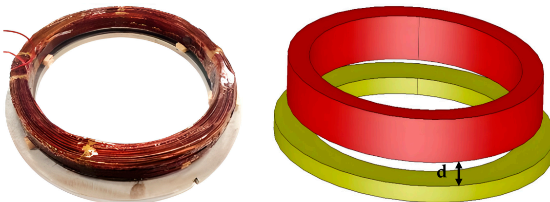
Figure 11. Experimental bench from bottom to top: the clamping plate and the circular inductor.
