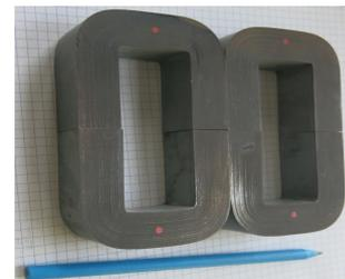
Fig. 1. wound core made with thin GOES strips.
