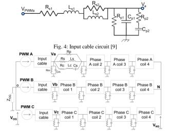
Fig. 5: Equivalent circuit for the electrical machine (first scale model) [10]
