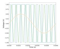
Fig. 3: Comparison between triangular and sinusoidal signal for PWM
