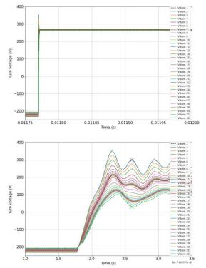
Fig. 9: a) Turn voltages with the steady state b) Turn voltages during the transient part
