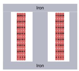
Fig. 1: Elementary coil in stator tooth
