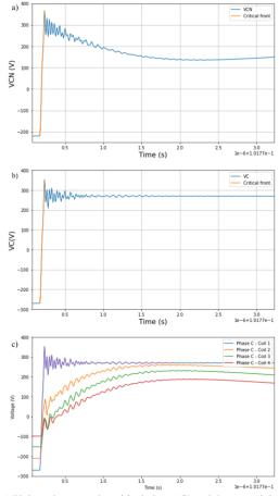
Fig. 7: a) Voltage between the critical phase (C) and the neutral during the critical edge, b) Voltage between the critical phase (C) and the ground during the critical edge, c) Distribution of the voltage between coils and ground during the critical edge
