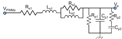
Fig. 4: Input cable circuit [9]
