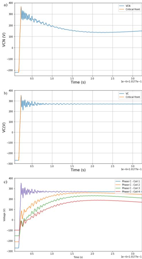
Fig. 7: a) Voltage between the critical phase (C) and the neutral during the critical edge, b) Voltage between the critical phase (C) and the ground during the critical edge, c) Distribution of the voltage between coils and ground during the critical edge
