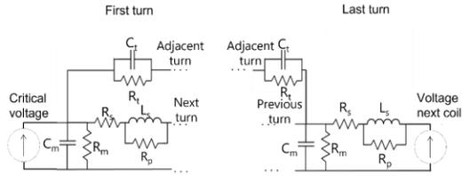
Fig. 8 :Turn equivalent circuit from [11]
