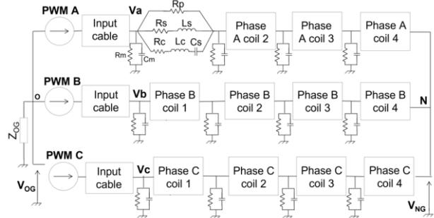
Fig. 5: Equivalent circuit for the electrical machine (first scale model) [10]
