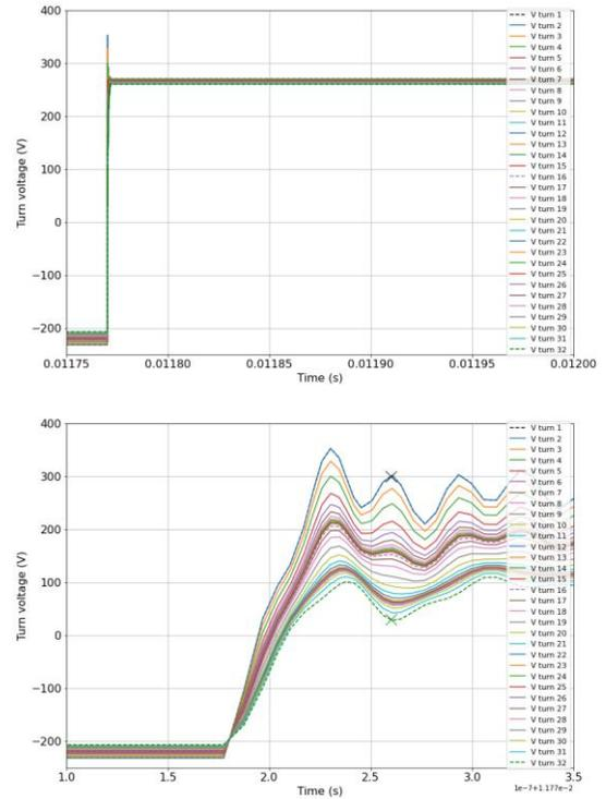
Fig. 9: a) Turn voltages with the steady state b) Turn voltages during the transient part
