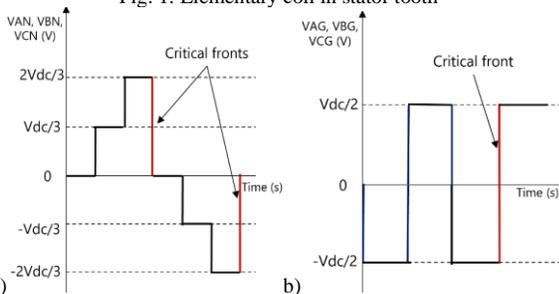
Fig. 2: a) Determination of the critical edge of the voltage between the phase and the neutral ( $V_{XN}$ ) for a perfect PWM, b) Determination of the critical edge of the voltage between the phase and the ground ( $V_{XG}$ ) for a perfect PWM
