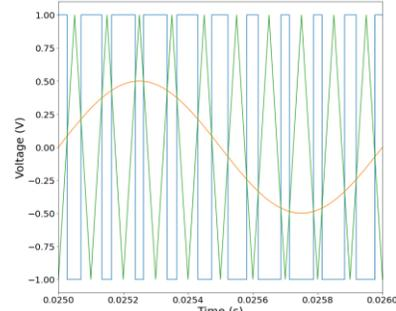
Fig. 3: Comparison between triangular and sinusoidal signal for PWM
