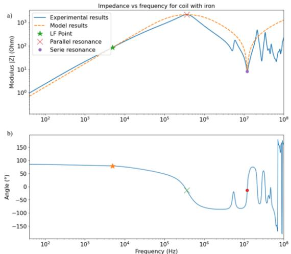
Fig. 6: Impedance measurements vs frequency done with an impedance analyzer for the determination of the parameters of the first scale model: a) the modulus, b) the phase
