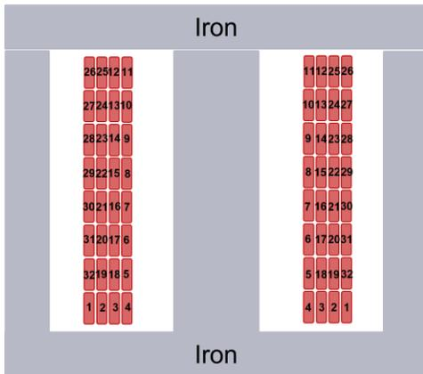
Fig. 1: Elementary coil in stator tooth
