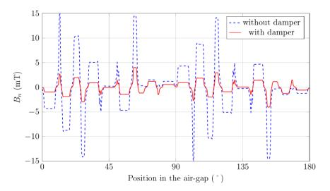
Fig.7. Normal flux density in the air-gap without (dashed line) and with (solid line) damper windings as a function of the position for f = 3100Hz and  $2\mu$ F capacitors.
