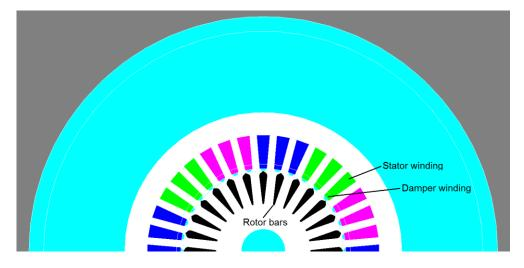
Fig.5. Used geometry of the 4kW induction machine with damper windings for FEM simulation (Flux2D).
