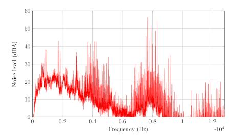
Fig.8. Noise level spectrum without damper windings for  $f_{PWM} = 4$ kHz.
