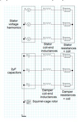
Fig.6. Coupling circuit of the 4kW induction machine with damper windings for FEM simulation (Flux2D).
