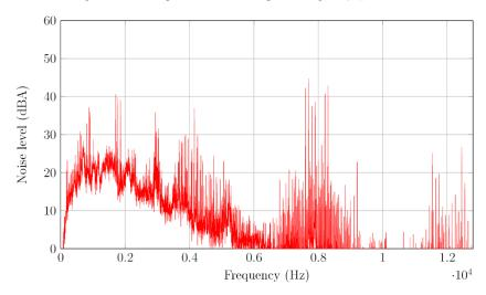
Fig.9. Noise level spectrum with damper windings for  $f_{PWM} = 4$ kHz and  $4\mu$ F capacitors.
