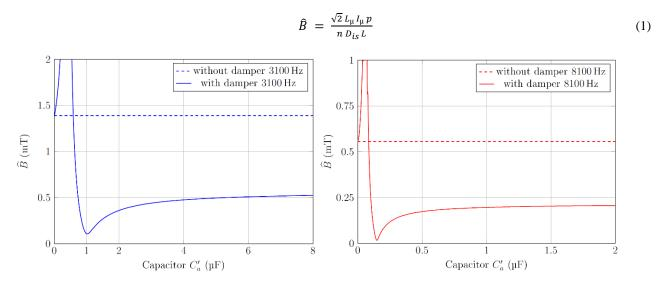
Fig.3. Peak flux density in the air-gap with (solid line) and without (dashed line) damper windings as a function of the capacitor  $C'_{\alpha}$  for f = 3100Hz and 8100Hz.
