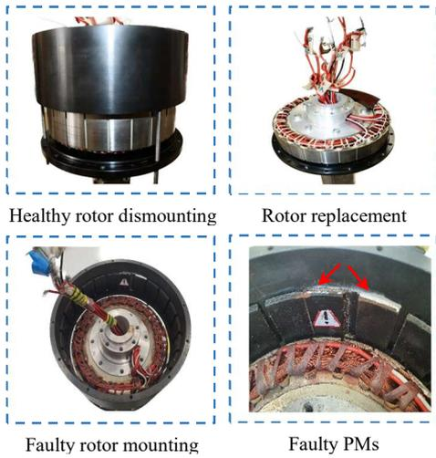
Fig. 19. Faulty rotor mounting of ER-PMSM prototype.
