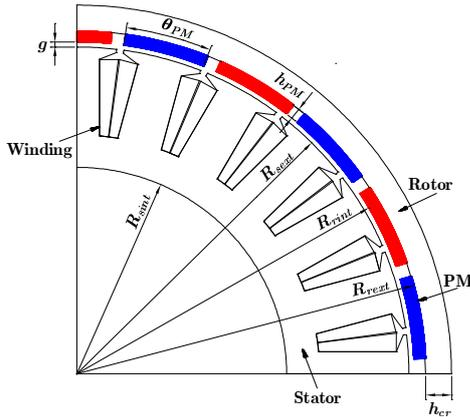
Fig. 1. Geometric parameters of the FSCW ER-PMSM.
