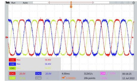
Fig. 21. The experimental healthy back-EMF of the ER-PMSM.
