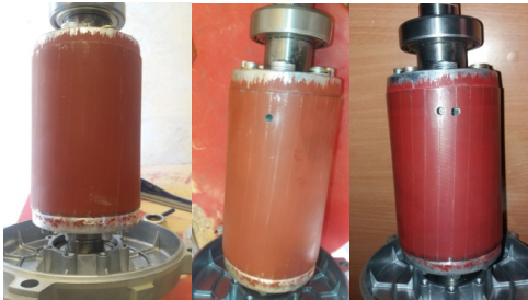
Figure 2. Photos of healthy and faulty rotor bars
