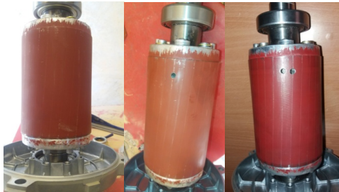
Figure 2. Photos of healthy and faulty rotor bars
