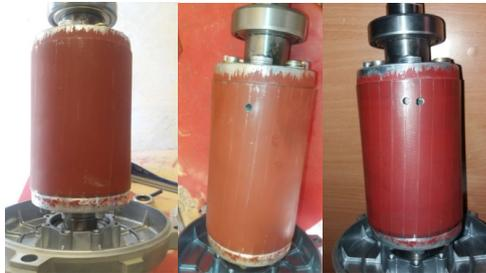
Figure 2. Photos of healthy and faulty rotor bars
