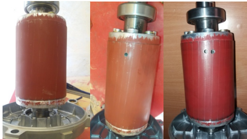
Figure 2. Photos of healthy and faulty rotor bars
