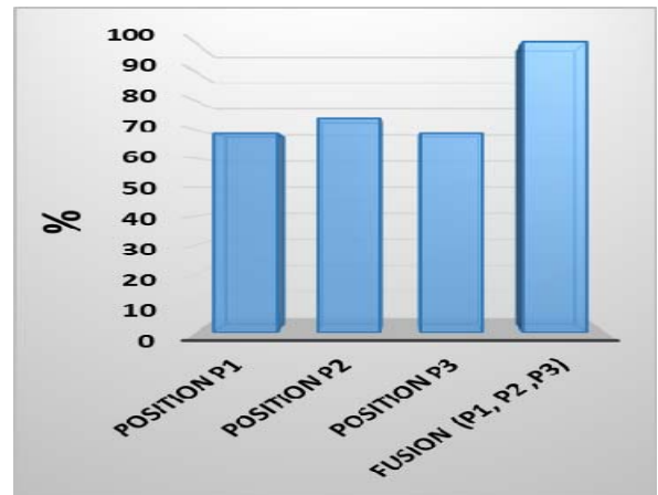
Fig. 5. Effect of the number of positions on the effectiveness of fault detection.
