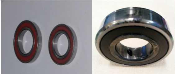
Fig.3. Picture of healthy and artificial inner raceway fault
