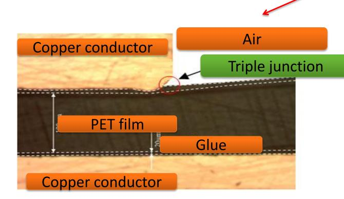
The breakdown voltage tests performed on the dielectric are rather promising : •9.5 kV AC for 100µm on the surface. •2.5 kV AC for100 µm on the edges.
