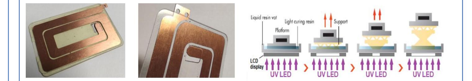
An alternative manufacturing process (patent application filed) is to use additive manufacturing, which consists of 3D printing successive layers using SLA – LCD technology on each face of the conductor. Well suitable for flat busbar (example : conductors for power planar transformer):
