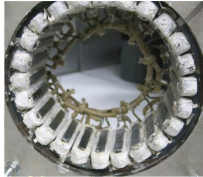
Fig. 1. Stator of a  $\text{HT}^{\circ}$  PMSM made with 24 rigid inorganic coils. The picture was made before closing the slots with metallic wedges.
