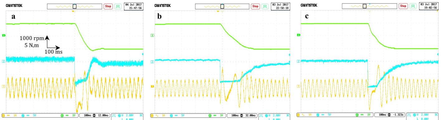
Fig.7 Rotation reversing maneuver: Rotor speed [rpm], Torque [N.m], Stator phase current [A].
