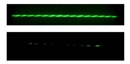
**Figure 5:** PDs pictures in both twisted pairs under identical voltages. Upper picture: standard enameled wire. Lower picture: enameled wire with the external semi-conductive layer.
