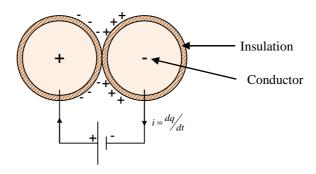
Figure 1: Diagram of partial discharge current formation in twisted pair.
