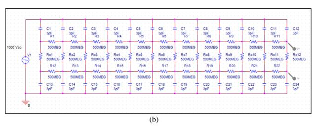
**Figure 6:** Equivalent circuit of a twisted pair with semi-conductive external layer.
