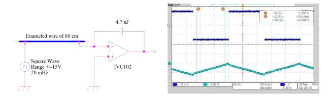
**Figure 7:** Simplified diagram of the low current measurement.
