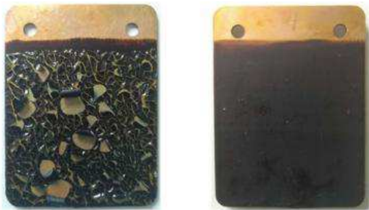
VILB varnish coated specimens after thermal ageing - Silane free (left), with silane (right).
