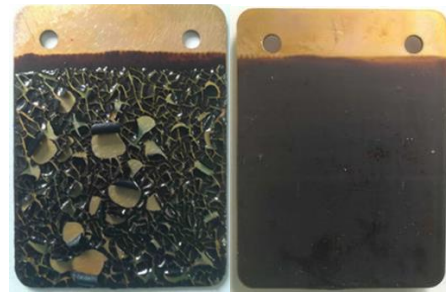
Fig. 2. Thermal withstanding improvement using 120 \mu m layer of varnish filled with 2%wt of Silane and 10%wt of Silica (Right) compared to unfilled varnish (Left) at 200 ^{\circ} C after 8h.
