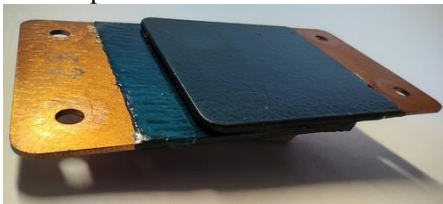
Fig. 1. Varnish Insulated Busbar (VIB) sample
