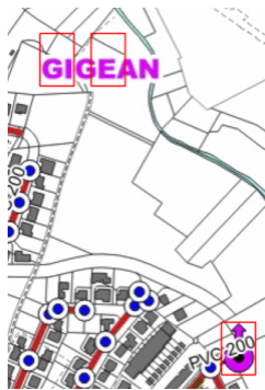
Fig. 9: False positive example with NCC on lifting station
