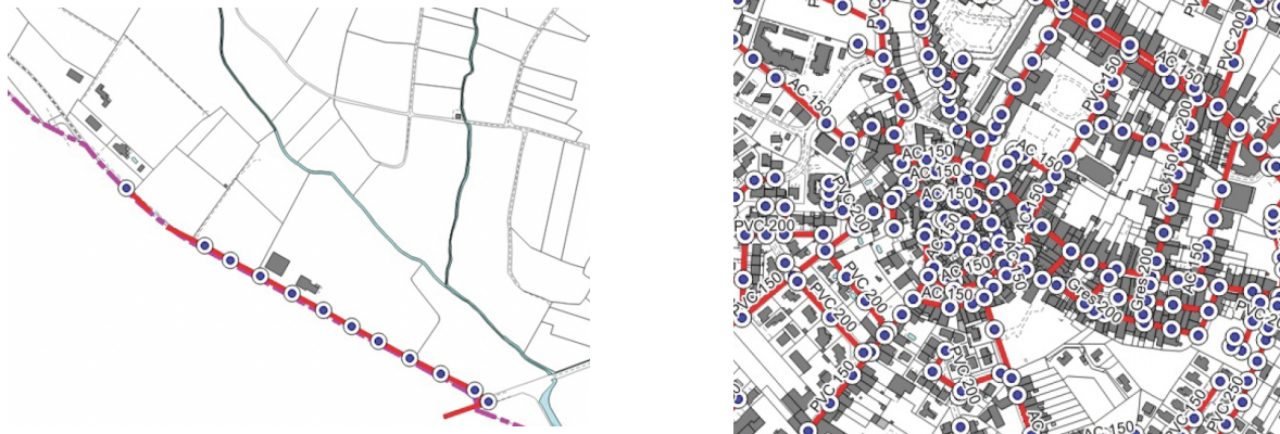
(a) A sub-image of the Gigean map (Figure 1) representing distant and independent manholes
