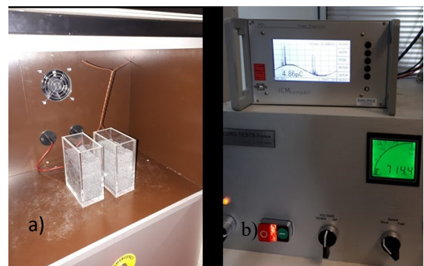
Figure 2 Electrical characterization devices: a) Breakdown voltage measurement, b) PDIV measurement.
