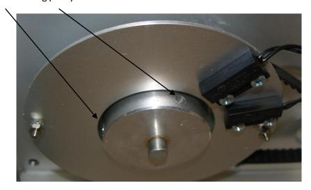
Insert an ohm-meter into terminal 1 and 3, thus rotate by hand the timing pulley, till an open circuit is shown on ohm-meter, at this point fix the two timing pulley screws, keep in tension the timing belt and fix its support.
