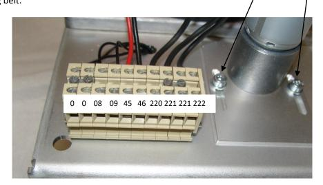
Set the variac brush to zero. Loose two screws of timing pulley
