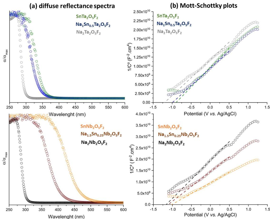
**Figure 4:** (a) diffuse reflectance spectra and (b) *Mott-Schottky plots* of  $\text{Na}_{2-2x}\text{Sn}_x\text{Ta}_2\text{O}_5\text{F}_2$  (top panels) and  $\text{Na}_{2-2x}\text{Sn}_x\text{Ta}_2\text{O}_5\text{F}_2$  (bottom panels).
