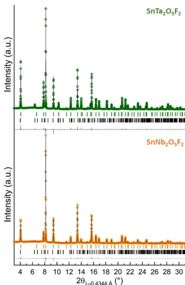
**Figure 2:** Rietveld refinement of the structures against synchrotron XRD data. The orange ( $\text{SnNb}_2\text{O}_5\text{F}_2$ ) and green ( $\text{SnTa}_2\text{O}_5\text{F}_2$ ) dots correspond to the experimental diffraction patterns, the black curves are the calculated diffraction patterns and the grey curves are the difference plots. The black tick marks indicate Bragg peaks of the  $\text{Nb}_2\text{O}_5$  (<1 w%) or  $\text{Ta}_2\text{O}_5$  (<5 w%) impurities.
