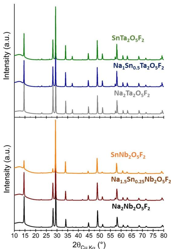
**Figure 1:** XRD patterns of the  $\text{Na}_{2-2x}\text{Sn}_x\text{M}_2\text{O}_5\text{F}_2$  compounds obtained by ion exchange synthesis from the pyrochlore  $\text{Na}_2\text{M}_2\text{O}_5\text{F}_2$  ( $M=\text{Nb}$  or  $\text{Ta}$ ).
