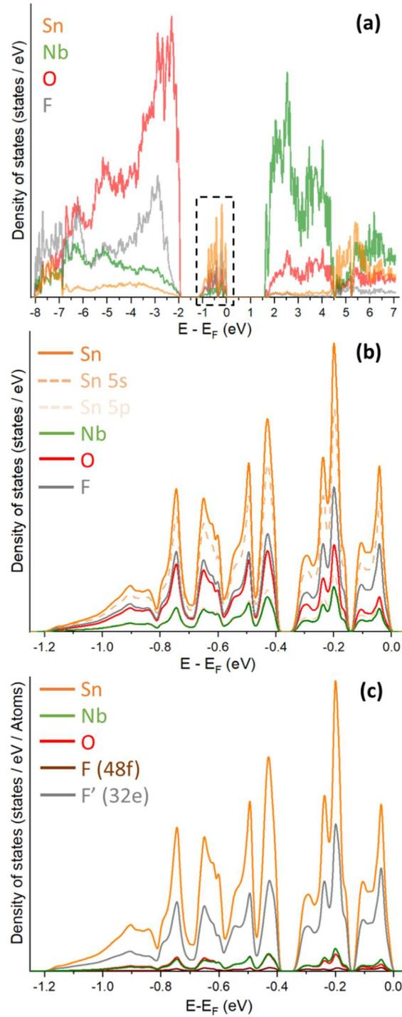
**Figure 5:** (a) PDOS of SnNb<sub>2</sub>O<sub>5</sub>F<sub>2</sub> with (b) the enlargement of the [-1.2 eV – 0 eV] region mainly composed of Sn 5s – (O,F) 2p – Sn 5p hybridized states and (c) the contributions to this region of the different crystallographic sites showing that X' anion (F, 32e site) more strongly overlap with Sn orbitals than X anions (O/F, 48f site).
