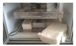
Figure 3- Thermal characterization device for building materials
