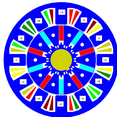
Fig. 2. Permanent magnet configuration
