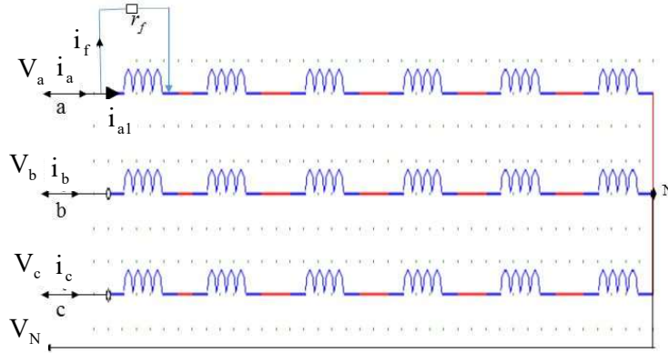
Fig.5. Faulty SPMSM model.
