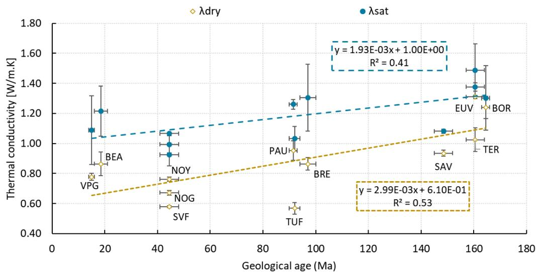
Fig. 9 Thermal conductivity as a function of geological age
