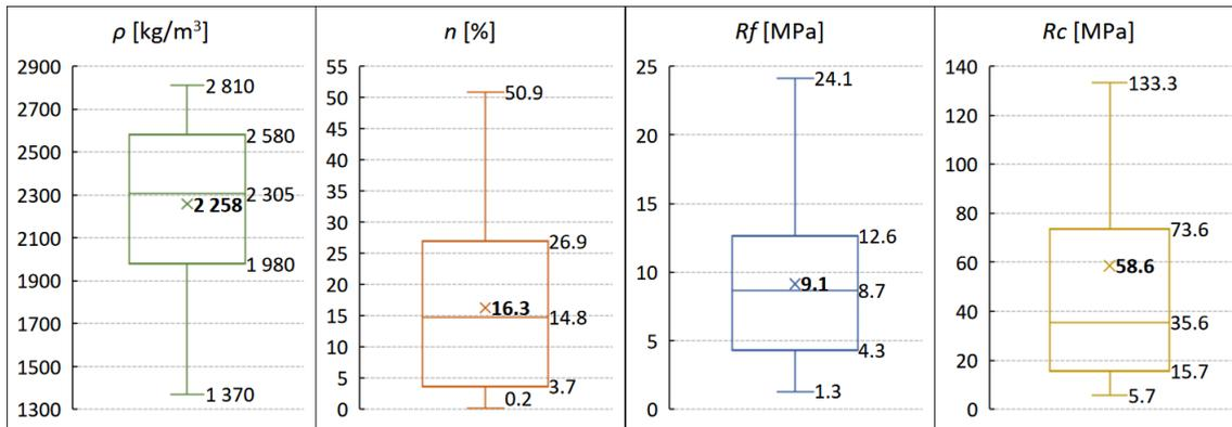
**Fig. 1** The extent of mechanical properties of limestone
