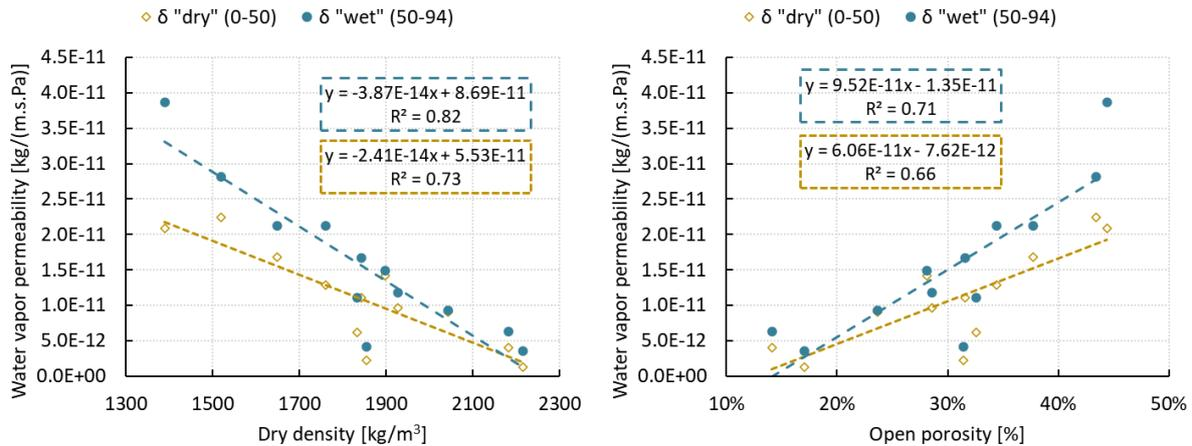
**Fig. 13** Water vapor permeability as a function of density, and open porosity
