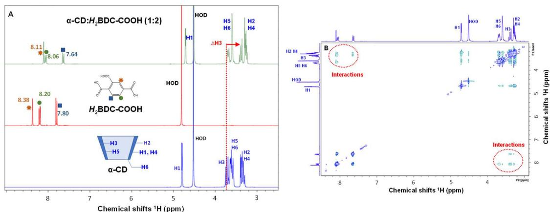
**Figure 4.** (A) NMR spectra (400 MHz, 25°C, D<sub>2</sub>O, 1 mM) of  $\alpha$ -CD (blue spectrum),  $H_2$ BDC-COOH (red spectrum) and 1/1 mixture of  $\alpha$ -CD and  $H_2$ BDC-COOH (green spectrum). (B) Partial contour plot of the T-ROESY spectrum of a D<sub>2</sub>O solution containing  $\alpha$ -CD and  $H_2$ BDC-COOH at the same concentration (1 mM).
