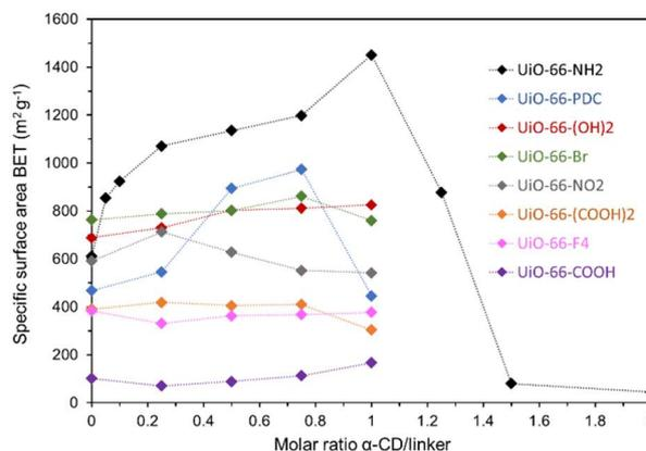
**Figure 1.** BET specific surface area as a function of the  $\alpha$ -CD/linker molar ratio used during the hydrothermal synthesis of the UiO-66-type MOFs. From the bottom to the top, UiO-66-COOH (purple), UiO-66-F<sub>4</sub> (pink), UiO-66-(COOH)<sub>2</sub> (orange), UiO-66-NO<sub>2</sub> (grey), UiO-66-Br (green), UiO-66-(OH)<sub>2</sub> (red), UiO-66-PDC and UiO-66-NH<sub>2</sub> (black).
