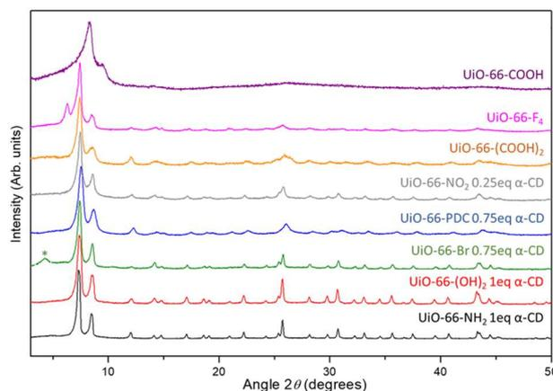
**Figure 3.** XRD patterns of the selected UiO-66-R materials synthesized using the selected molar ratio of  $\alpha$ -CD with respect to the linker. The star symbol is assigned to the reo defect phase.
