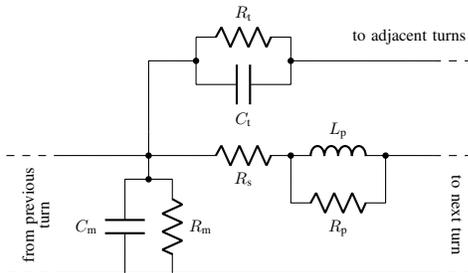
Fig. 2. Lumped parameter equivalent circuit of one turn.
