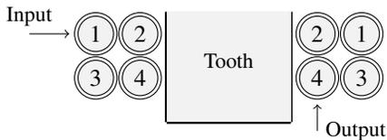
Fig. 3. An example of a 4-turn winding.
