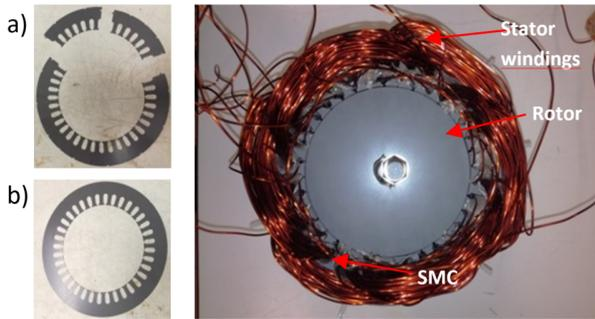
**Figure 2:** Implementation stack with an example of a) segmented and b) non-segmented sheet
