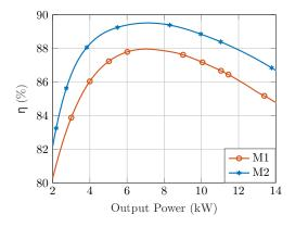
Fig. 14. Efficiency according to IEC60034-2-1
