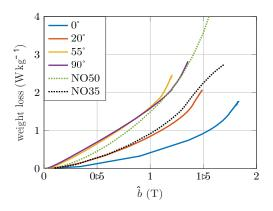
Fig. 6. Core losses for each  $\hat{b}(\hat{h})$  curve
