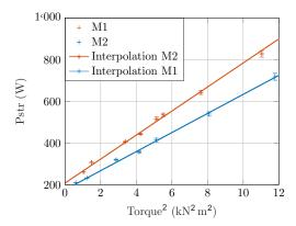
Fig. 13. Stray load losses
