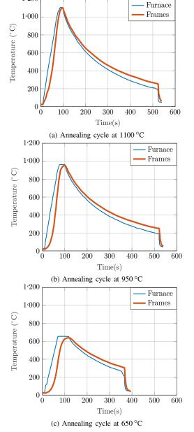
Fig. 2. Annealing cycle on Epstein Frame
