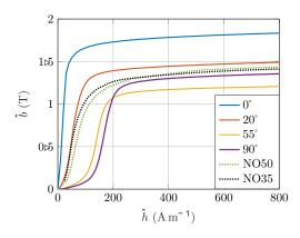
Fig. 5.  $\hat{b}(\hat{h})$  curves for different materials and different angle  $\alpha$
