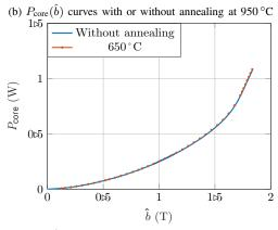
(c)  $P_{\text{core}}(\hat{b})$  curves with or without annealing at 650 °C
