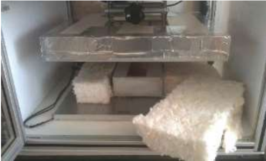
Figure 3- Thermal characterization device for building materials
