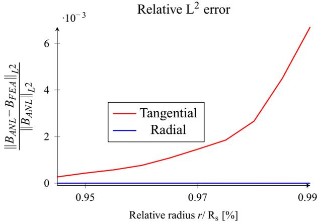
**Figure 5:** Comparison between analytical (ANL) and numerical (FEA) computations of the magnetic flux density components  $B_r$  and  $B_t$  depending on the radius with a slotless machine for a wave-number  $k = 2$ .
