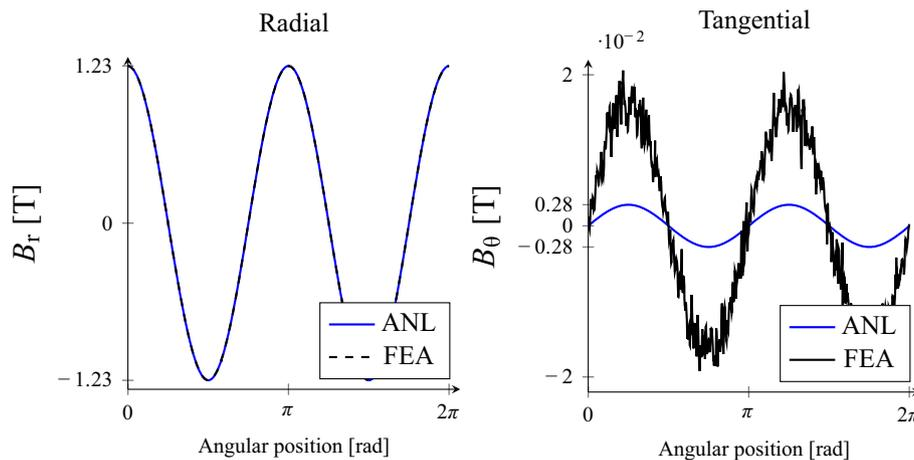
**Figure 4:** Comparison between analytical (ANL) and numerical (FEA) computations of the magnetic flux density components  $B_r$  and  $B_t$  at radius  $r = 0.9996R_s$  with a slotless machine for a wavenumber  $k = 2$ .
