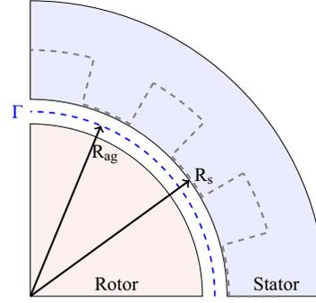
Figure 2: Illustration of the air-gap Maxwell tensor application.
