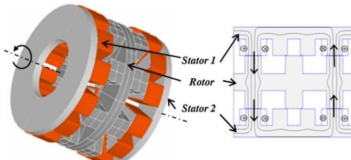
Fig. 1 Flux path (transverse loop)
