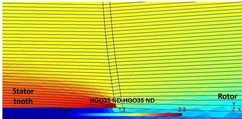
Fig. 12 Flux lines distribution for  $HGO_{35}^{ND}$ - $HGO_{35}^{ND}$
