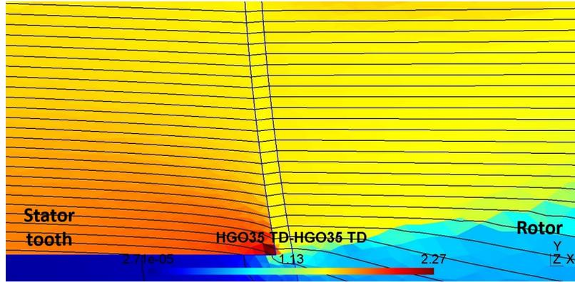
Fig. 11 Flux lines distribution for  $HGO_{35}^{TD}$ - $HGO_{35}^{TD}$
