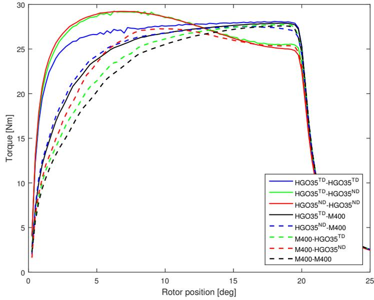
**Fig. 14** Torque variations with rotor position at 0.8A
