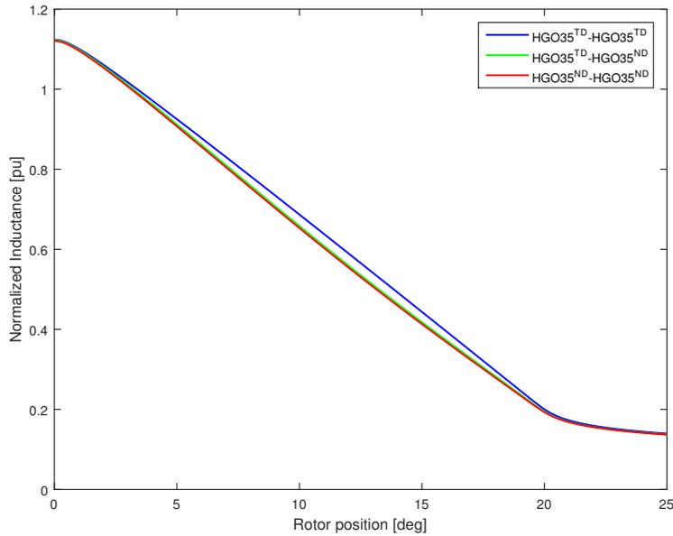
**Fig. 7** Inductance for 3 anisotropic cases at 0.8A
