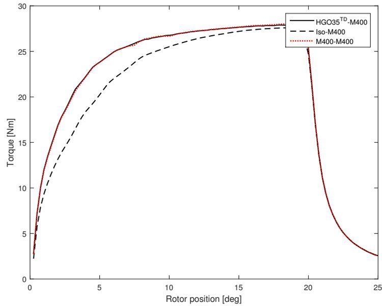
Fig. 13 Influence of anisotropy on the electromagnetic torque
