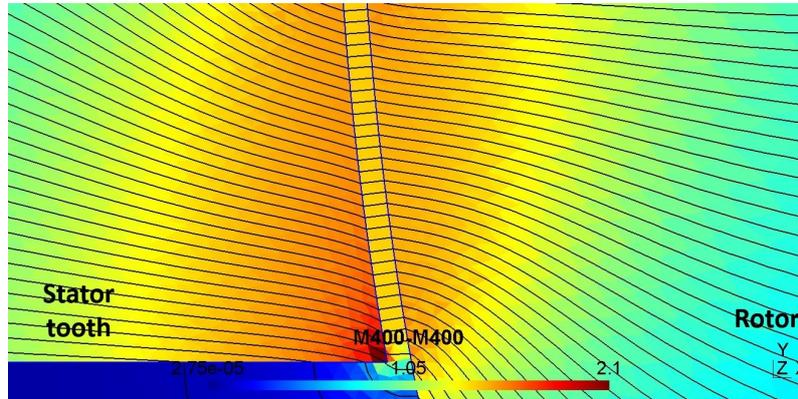
**Fig. 8** Flux lines distribution for M400-M400
