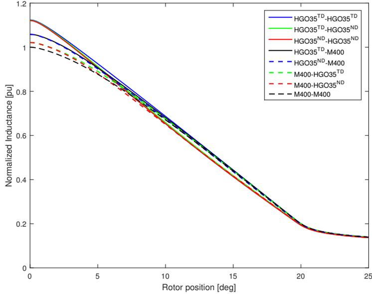
**Fig. 6** Inductance variations with rotor position at 0.8A
