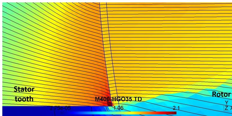
**Fig. 10** Flux lines distribution for M400- $HGO_{35}^{TD}$
