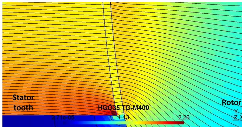
**Fig. 9** Flux lines distribution for  $HGO_{35}^{TD}$ -M400
