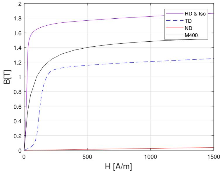
**Fig. 4** B(H) curves in the numerical model
