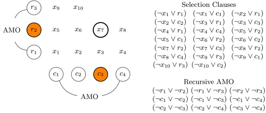
**Fig. 1.** Encoding the AtMost-1 constraint  $\sum_{i=1}^{i \leq 10} x_i \leq 1$  with the two product encoding, and two auxiliary AtMost-1 constraints  $r_1 + r_2 + r_3 \leq 1$  and  $c_1 + c_2 + c_3 + c_4 \leq 1$ .
